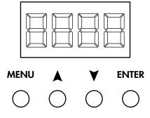
The Control Display shows the current state of the unit. It is used to select the operating mode, as well as the sub-features. For detailed functions, please see the section below.
